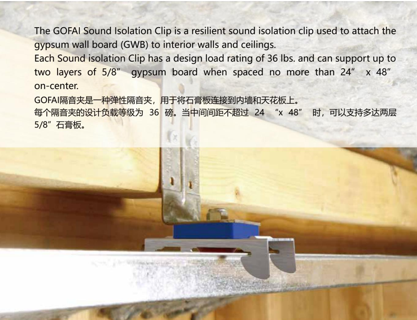
This section describes the elastic sound insulation clamps mounted on plasterboard grooves that support plasterboard, wood, concrete, etc., for wall and ceiling sound insulation (separation coupling).
